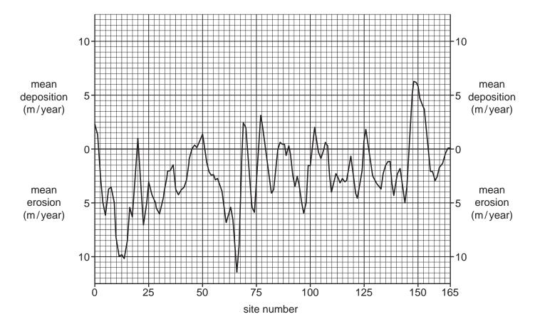
Mean erosion and mean deposition rates along a stretch of coastline on Hatteras Island, North Carolina, USA, 1989–2002
